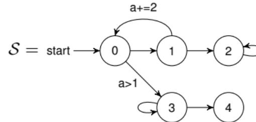
A finite set of path schemas fully describes all runs in the flat system  $\mathcal{S}$ :
